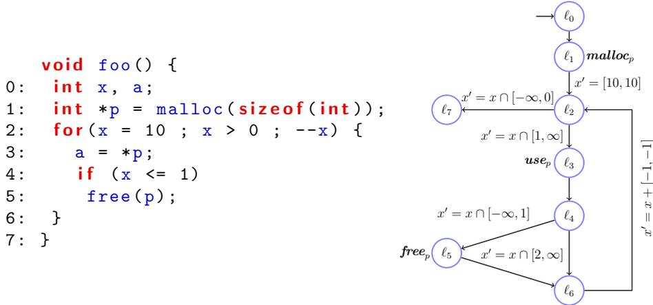
Fig. 1. Example program and the generated CFG with annotations, and generated interval equations for variable  $x$ . The annotated CFG is used for model checking, the interval equations for abstract data tracking.
